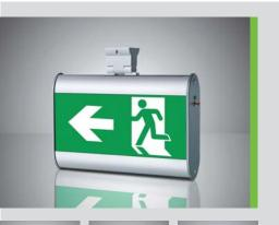
Single- or double-sided Anodized aluminum case Polycarbonate side cover and hanger SMD LED application Charge and battery capacity status display with green LEDs High-temperature Ni-Cd battery cells Overcharge and deep discharge protection White acrylic plate Back lighting Ceiling mounted or wall mounted Optional - 110 VAC compatibility Optional - Metal hanger, hook or steel wire
