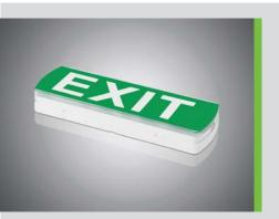
Indoor use Polycarbonate case and glass SMD LED application High energy saving Long life-time (50.000 hours) Emergency lighting function by interruption of the unswitched phase 3 hours duration in case of emergency Charge status display with green LED High-temperature Ni-Cd battery cells Overcharge and deep discharge protection Ceiling or wall mounted
