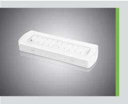
Indoor use Polycarbonate case and glass SMD LED application High energy saving Long life-time (50.000 hours) Emergency lighting function by interruption of the unswitched phase 3 hours duration in case of emergency Charge status display with green LED High-temperature Ni-Cd battery cells Overcharge and deep discharge protection Ceiling or wall mounted
