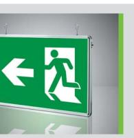
Single- or double-sided Anodized aluminum case Polycarbonate side cover and hanger SMD LED application Status display with green and red LEDs Test switch Remote control and test with DALI interface High-temperature Ni-Cd battery cells Overcharge and deep discharge protection White acrylic plate Back lighting Ceiling mounted, ceiling recessed or wall mounted Optional - 110 VAC compatibility Optional - Metal hanger, hook or steel wire Optional - LiFePO4 or Ni-MH battery application
