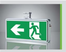
Single- or double-sided Anodized aluminum case Polycarbonate side cover and hanger SMD LED application Charge status display with green LED Test switch High-temperature Ni-Cd battery cells Overcharge and deep discharge protection White acrylic plate Back lighting Ceiling mounted, ceiling recessed or wall mounted Optional - 110 VAC compatibility Optional - Metal hanger, hook or steel wire
