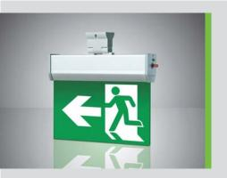
Single- or double-sided Anodized aluminum case Polycarbonate side cover and hanger SMD LED application Charge and battery capacity status display with green LEDs High-temperature Ni-Cd battery cells Overcharge and deep discharge protection Transparent plexiglas with screen printed Side lighting Ceiling mounted, ceiling recessed or wall mounted Optional - 110 VAC compatibility Optional - Metal hanger, hook or steel wire
