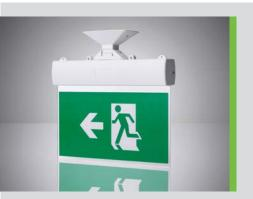
Single- or double-sided Polycarbonate case and hanger SMD LED application Charge and battery capacity status display with green LED High-temperature Ni-Cd battery cells Overcharge and deep discharge protection Transparent plexiglas with screen printed Side lighting Ceiling mounted, ceiling recessed or wall mounted
